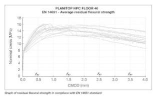
Typical residual flexural strength behaviour in compliance with EN 14651
